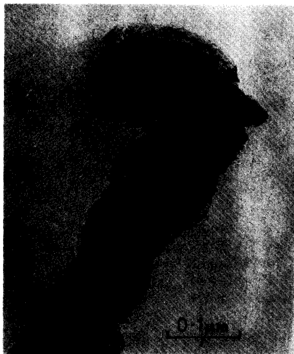
Fig. 6. Carbon filament formed in optical microscope at 700°C.
